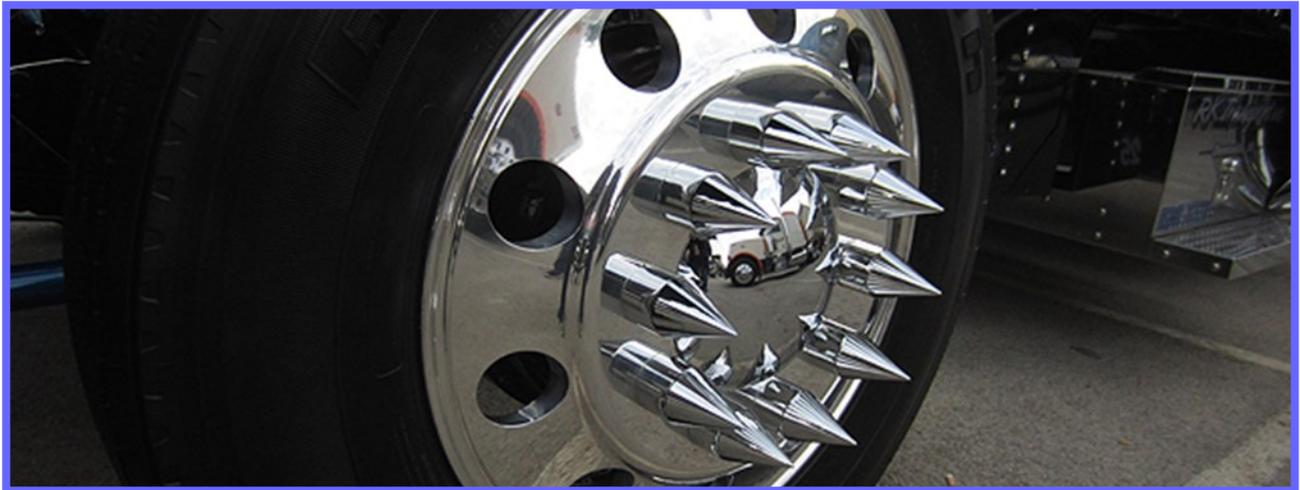
Neither the Australian Design Rules (ADRs) or Heavy Vehicle (Mass, Dimension & Loading) National Regulation (HV(MDL)NR) exclude wheel nuts from overall width measurement.
