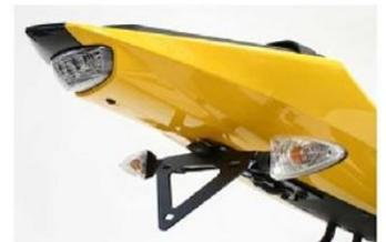
iv) a rear retro-reflector is fitted at no more than 15° from the vertical
