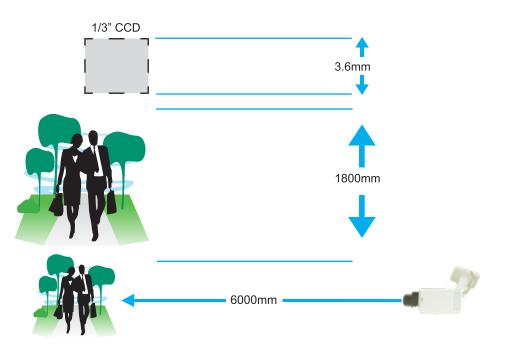
1/3" image sensor has a height of 3.6mm, divided by height of subject target of 1800mm and multiplied by distance from the camera at 6000mm.
